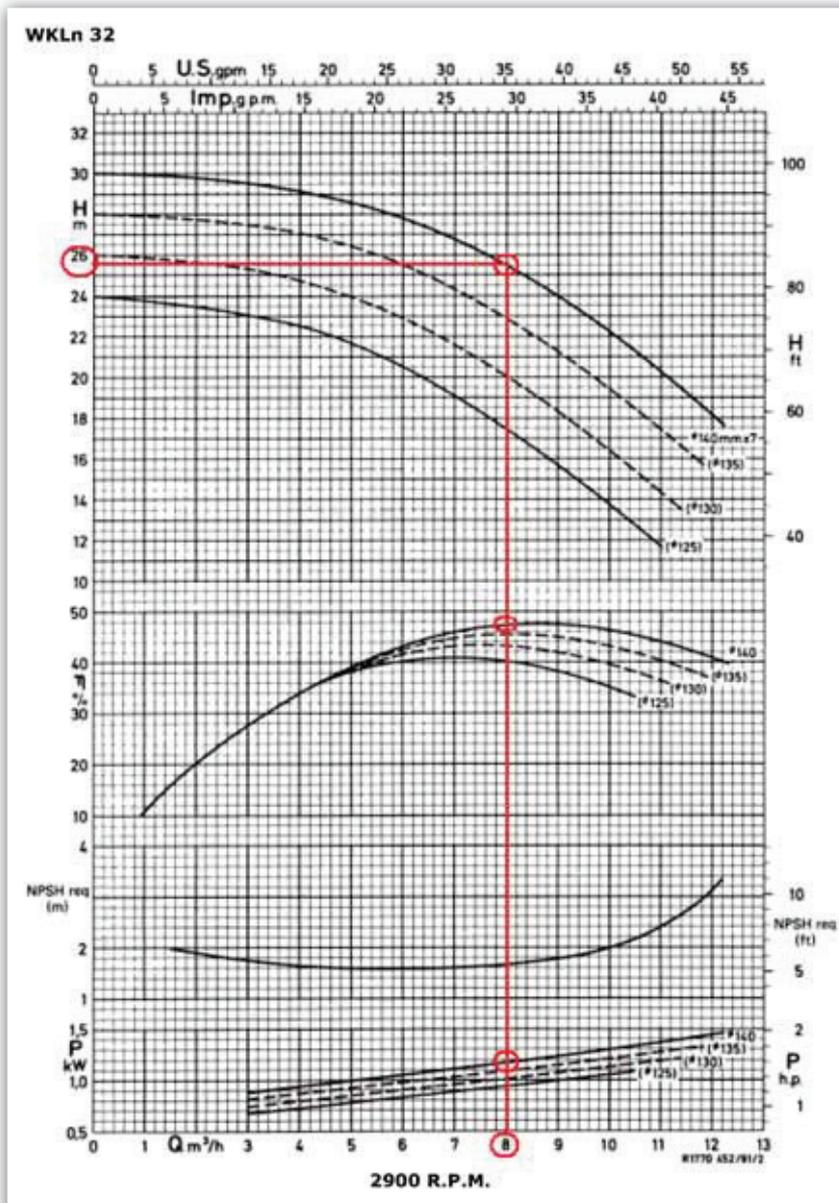
Figure 1. A pump curve for a KSB WKLn 32, 2 900 rpm pump. (<http://www.ksbpumps.co.za>)
